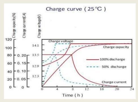
Lead Carbon Batteries are high-end products that work best with good quality battery chargers that have a compatible charge profile (or ability to adjust custom charge settings). Below settings for automated battery chargers are recommended to fully utilize the benefits of Lead Carbon Batteries.
